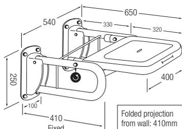
The 650mm projection shower seat is designed for use with a stainless steel backrest rail.
