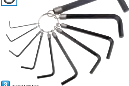
3 TKR10M/B 10 PIECE METRIC HEXAGON KEY SET Manufactured from hardened and tempered chrome vanadium steel. Each held on key ring holder. Display packed. Contents: 1.5, 2.0, 2.5, 3.0, 4.0, 5.0, 5.5, 6.0, 8.0 and 10mm
