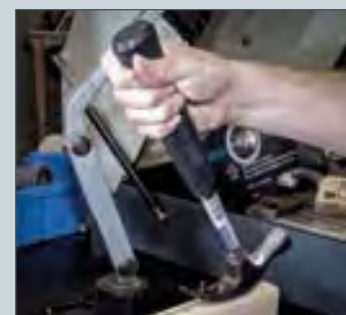
Nail extraction test for claw hammer
