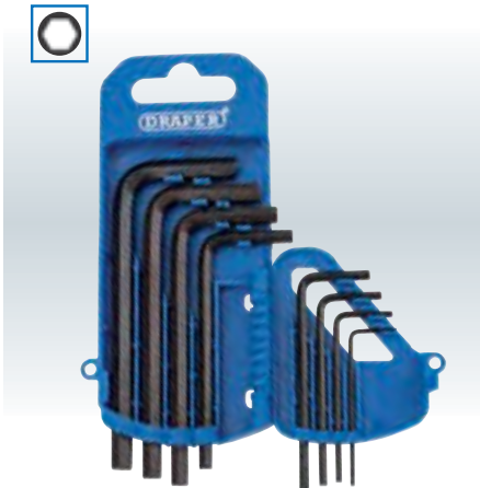
9 TKW8M/B 8 PIECE METRIC HEXAGON KEY SET Hexagon keys manufactured from hardened and tempered chrome vanadium steel. Held in plastic storage holder. Display packed. Contents: 1.5, 2.0, 2.5, 3.0, 4.0, 5.0, 5.5 and 6.0
