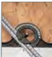
PROTRACTOR For measuring and marking angles.
