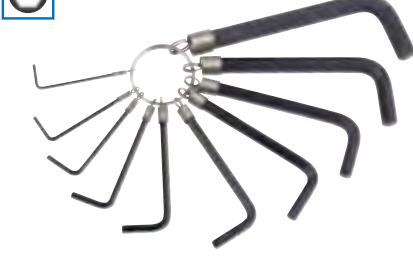
2 TKR10A/B 10 PIECE IMPERIAL HEXAGON KEY SET Manufactured from hardened and tempered chrome vanadium steel. Each held on key ring holder. Display packed. Contents: 1/16, 5/64, 3/32, 1/8, 5/32, 3/16, 7/32, 1/4, 5/16 and 3/8"
