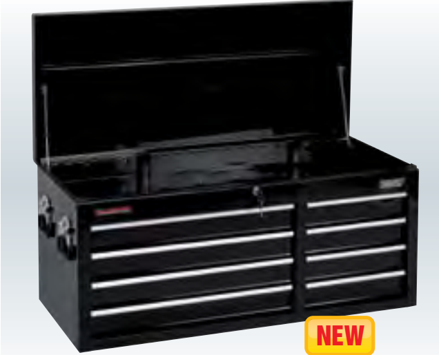
2 TC8B/40/BK 8 DRAWER 40" TOOL CHEST (BLACK) Eight drawer tool chest manufactured from sheet steel with a powder coated finish. All drawers are fitted with anti slip mats and ball bearing runners for smoother operation and longer life. Each tool chest is has a secure integral locking system supplied with two keys and heavy-duty carry handles. Carton packed. Drawer configuration: • 4 drawers: 569 x 400 x 75mm • 4 drawers: 300 x 400 x 75mm
