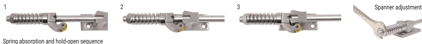
Spring absorption and hold-open sequence
